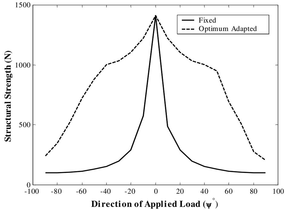
**Figure 3 :** Structural strength,  $S_s$ , versus the direction of the applied load for the fixed and optimized adapted structure under Static load.
