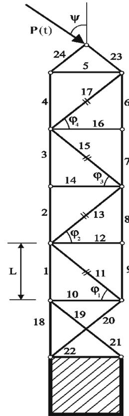
Figure 2 : The 24-bar plane adaptive truss structure with active members 11, 13, 15, and 17
