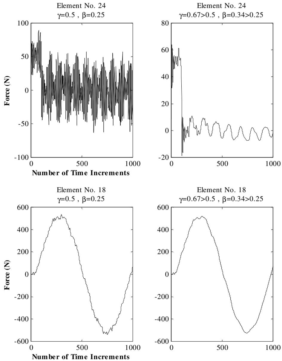
Figure 6 : Time histories of the element forces for case II and impact  $I_p = 1$  N-sec.
