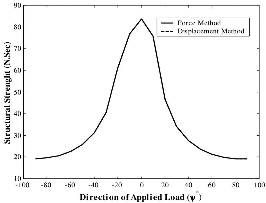
Figure 7 : Structural strength,  $S_d$ , versus the direction of the applied load for the fixed structure (Dynamic load).
