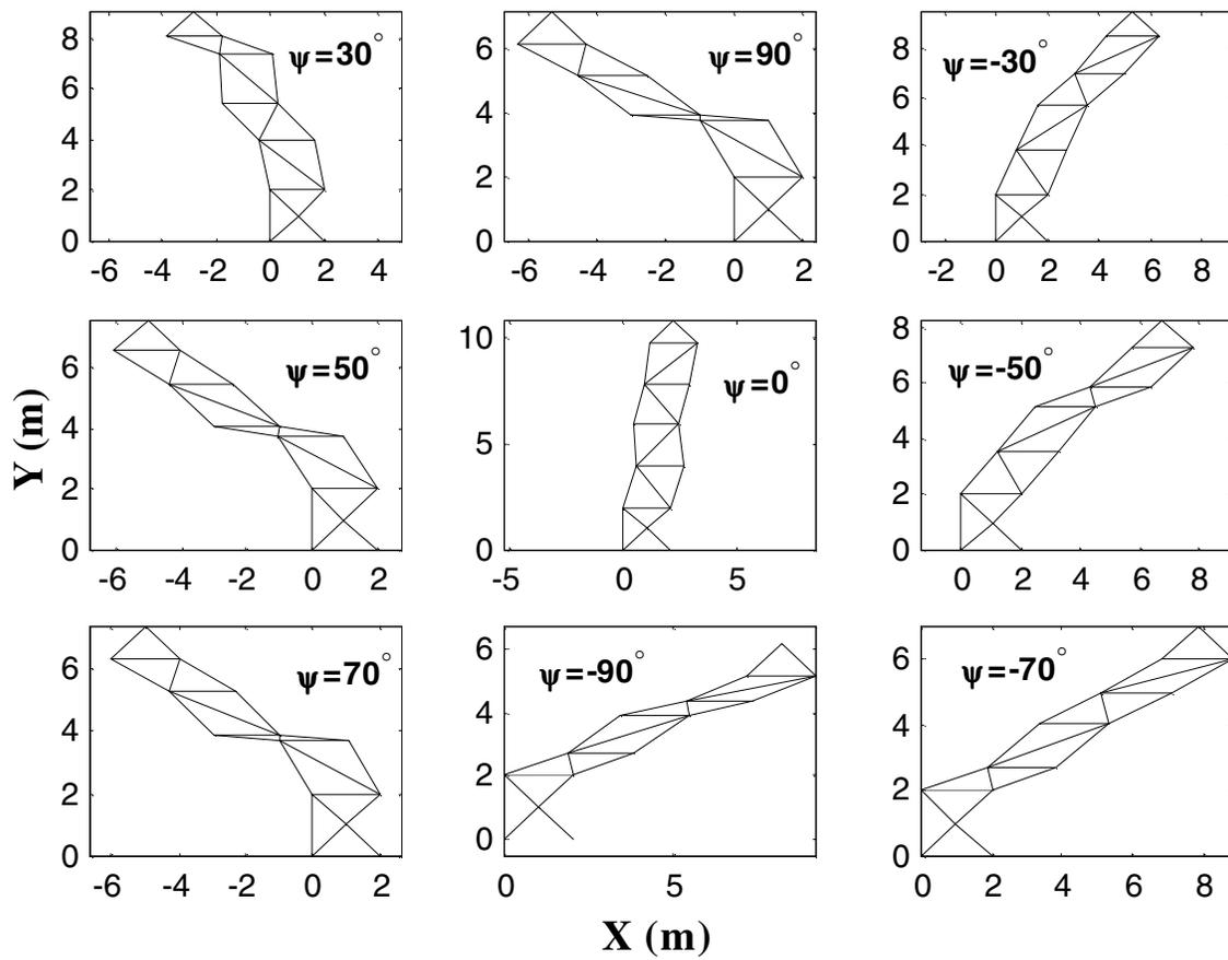
Figure 9 : Optimal adaptive shapes for dynamic load
