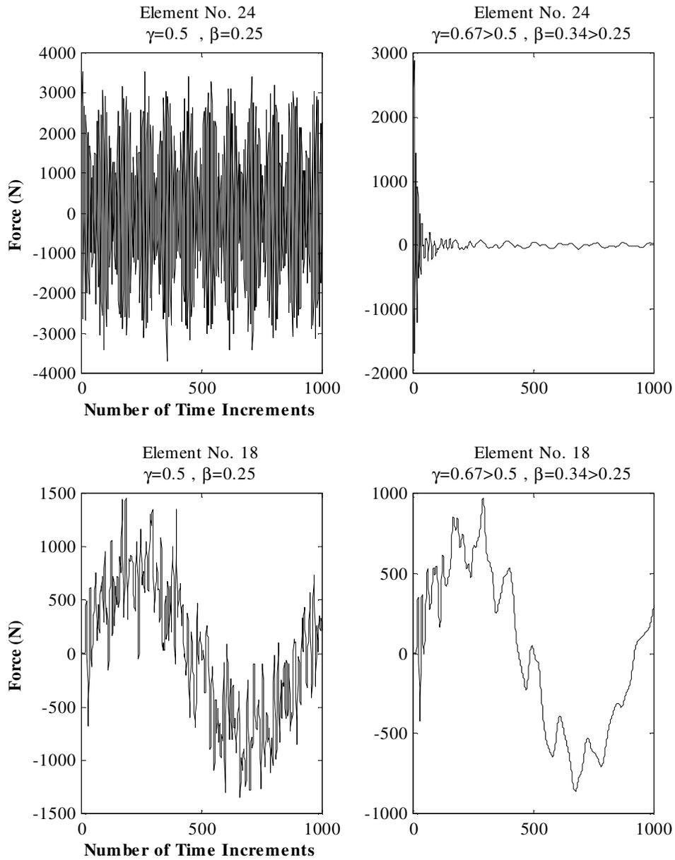
Figure 5 : Time histories of the element forces for case I and impact  $I_p = 1$  N-sec.
