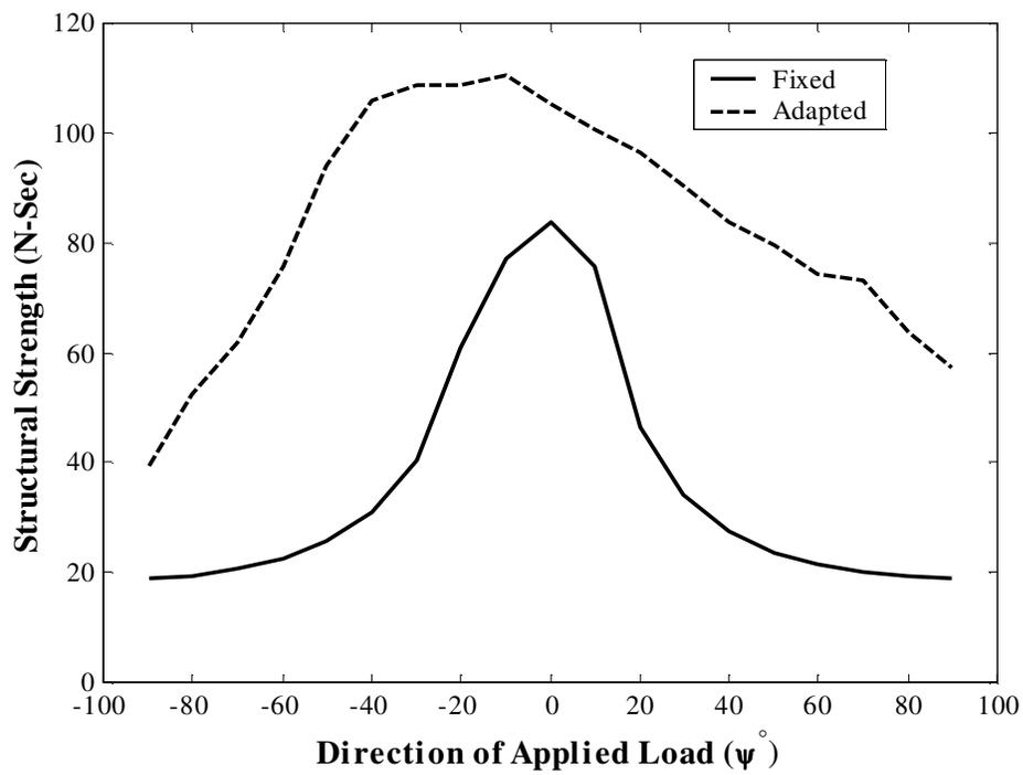
Figure 8 : Optimal adaptive and fixed structural strength versus the direction of the applied load (Dynamic load).
