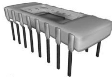
**Figure 18 :** Motorola package, shown in deformed view after simulation of the package at 200 °C
